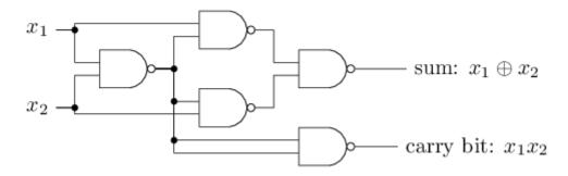
To get an equivalent network of perceptrons we replace all the NAND gates by perceptrons with two inputs, each with weight -2-2, and an overall bias of 33. Here's the resulting network. Note that I've moved the perceptron corresponding to the bottom right NAND gate a little, just to make it easier to draw the arrows on the diagram:
