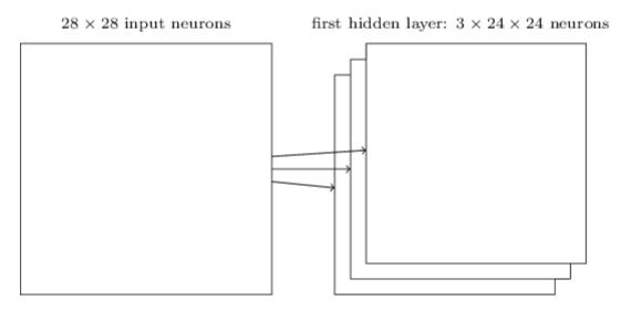
In the example shown, there are 33 feature maps. Each feature map is defined by a set of  $5 \times 55 \times 5$  shared weights, and a single shared bias. The result is that the network can detect 33 different kinds of features, with each feature being detectable across the entire image.
