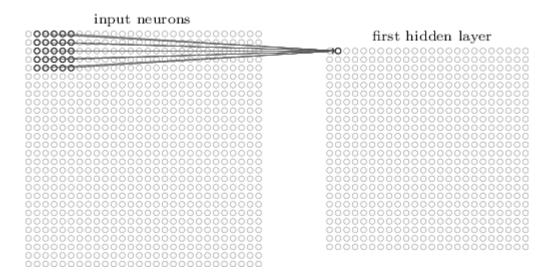
And so on, building up the first hidden layer. Note that if we have a 28×2828×28 input image, and 5×55×5 local receptive fields, then there will be 24×2424×24 neurons in the hidden layer. This is because we can only move the local receptive field 2323 neurons across (or 2323 neurons down), before colliding with the right-hand side (or bottom) of the input image.
