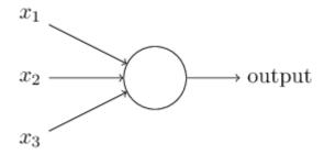
In the example shown the perceptron has three inputs, x1,x2,x3x1,x2,x3. In general it could have more or fewer inputs. Rosenblatt proposed a simple rule
