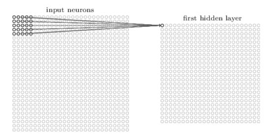
Then we slide the local receptive field over by one pixel to the right (i.e., by one neuron), to connect to a second hidden neuron:
