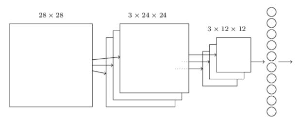
The network begins with 28×2828×28 input neurons, which are used to encode the pixel intensities for the MNIST image. This is then followed by a convolutional layer using a 5×55×5 local receptive field and 33 feature maps. The result is a layer of 3×24×243×24×24 hidden feature neurons. The next step is a max-pooling layer, applied to 2×22×2 regions, across each of the 33 feature maps. The result is a layer of 3×12×123×12×12 hidden feature neurons.
