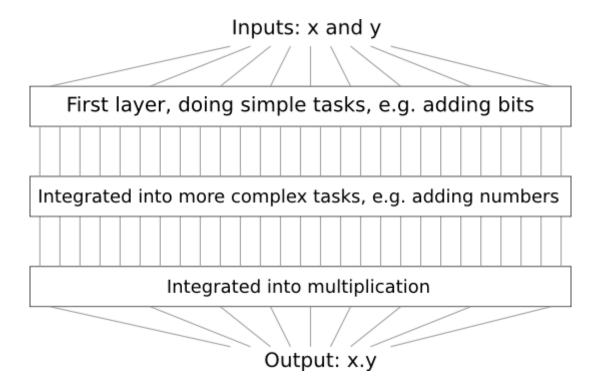
That is, our final circuit contains at least three layers of circuit elements. In fact, it'll probably contain more than three layers, as we break the sub-tasks down into smaller units than I've described. But you get the general idea.
