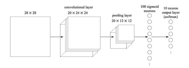
In this architecture, we can think of the convolutional and pooling layers as learning about local spatial structure in the input training image, while the later, fully-connected layer learns at a more abstract level, integrating global
